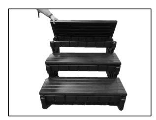
Step 4: Install the steps (finished edge out) by placing over the male lugs on the step sidewall and hitting downward with a rubber mallet. If the treads don't fully engage onto the lugs it may be necessary to step on the tread directly over the lugs and force down with your foot.
