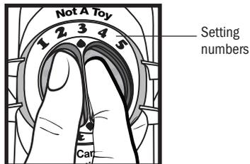
**4.** Twist the dial on the chlorine cartridge to the setting number for your pool size (see chart below).
