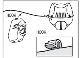
Do not remove the chlorine cartridge until the system has completely flipped. If the chlorine cartridge contains a small amount of chlorine after the system has flipped over, hang on the tether via the hook on the side of the cartridge until completely empty. Do not allow chlorine cartridge to sink to the bottom or pool bleaching may occur. When completely empty, discard in trash or offer for recycling.
