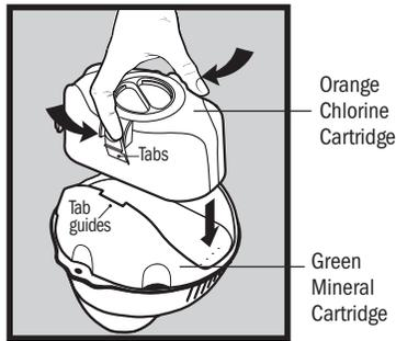
**3.** Remove outer packaging from both the mineral and chlorine cartridges of Flippin' FROG XL. Align the chlorine cartridge with tab guides on the mineral cartridge. Push together until you hear the cartridge click into place.
