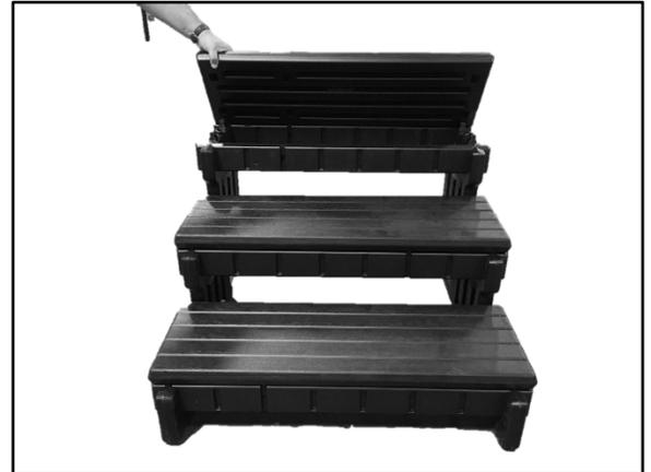
**Step 4:** Install the steps (finished edge out) by placing over the male lugs on the step sidewall and hitting downward with a rubber mallet. If the treads don't fully engage onto the lugs it may be necessary to step on the tread directly over the lugs and force down with your foot.
